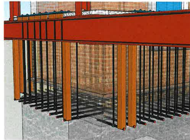
AT BOTTOM OF BRICK 2" HOLES WILL BE DRILLED THROUGH THE BUILDING WALLS SO THAT HORIZONTAL RODS CAN PASS THROUGH STRUCTURE.
